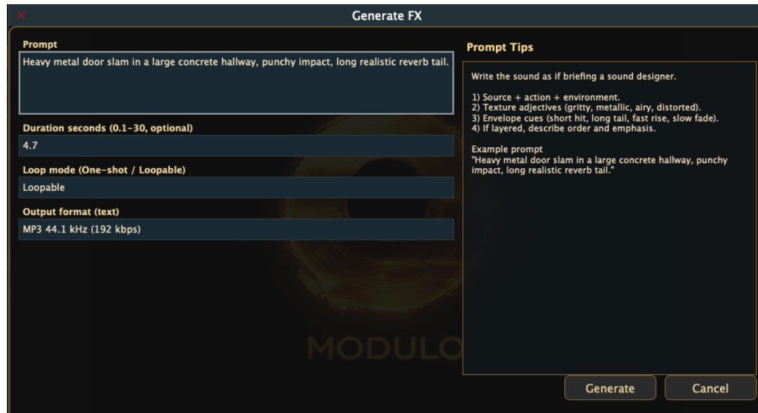
Figure 9.1: The Generate SFX dialog. Four primary controls, namely prompt, duration, loop mode, and prompt influence or output format, sit beside a rotating Prompt Tips sidebar that seeds the user’s mental model of what the model can produce. Generated audio is inserted at the playhead as a new clip with the originating prompt preserved as clip meta-data.
